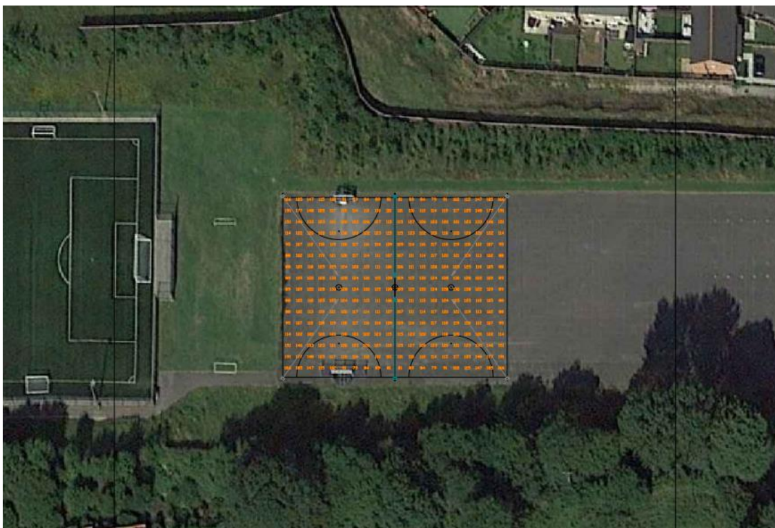
Figure 1 – Proposed siting of floodlights around MUGA facility
